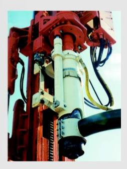
The percussion underreamer along with a small compact **Holte Casing Driver** Model 140, which also serves as a diverter, will allow the casing to be placed easily.
