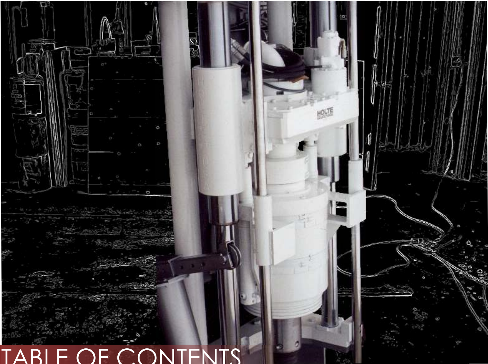
Casing Driver with Bearing Box (for Rigs with thrust bearing) mounted for underground mining.
