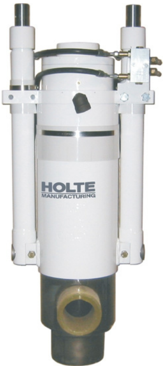
Holte Casing Driver 140 , is 45" tall (not including the cylinders) and has a 12" diameter. Weight is approximately 750 lbs. This casing driver is mounted under the top head of a drill rig.
