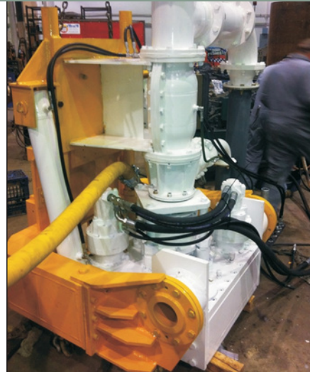
Reverse circulation (RC) TOP HEAD DRIVE with swivel and discharge elbow.
